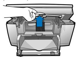
**3** Remove the cardboard insert from the inside of the unit.
